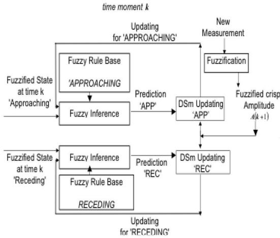
Figure 1: Block diagram of target's behavior tracking system
